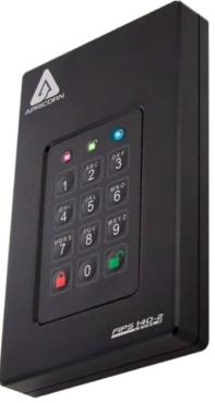
For the ultimate protection of your most sensitive data in storage and transportation, the Aegis Fortress L3 is designed and built to meet NIST FIPS 140-2 Level-3 requirements for the entire device. This complete FIPS validation includes the encryption module, all electronics, the hard drive, and the enclosure itself within the certification boundary.
